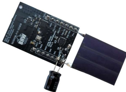
Batteryless LR NanoBeacon Using Energy Harvesting
